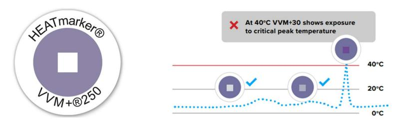
HEATmarker® VVM+ used in a Controlled Temperature Chain (CTC).
