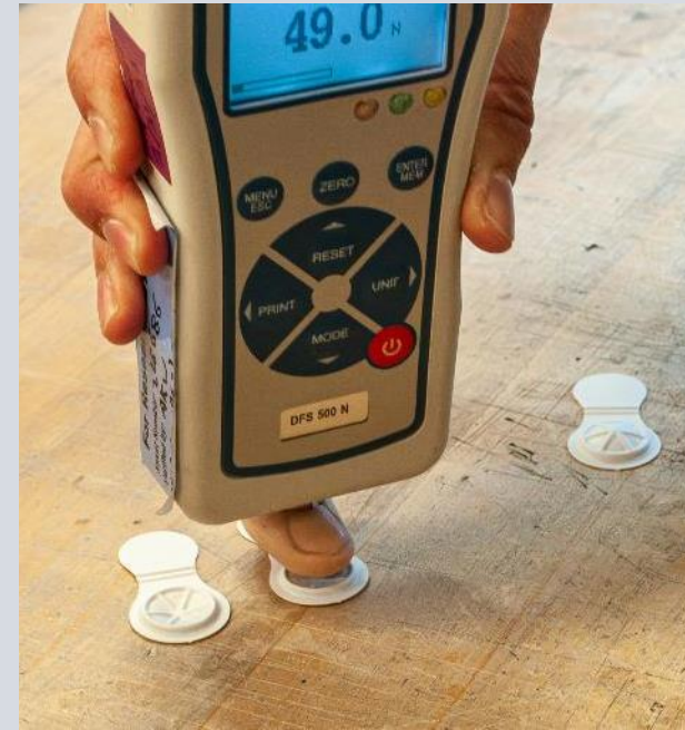
Different methods for force testing MAP feedback indicator prototypes.
