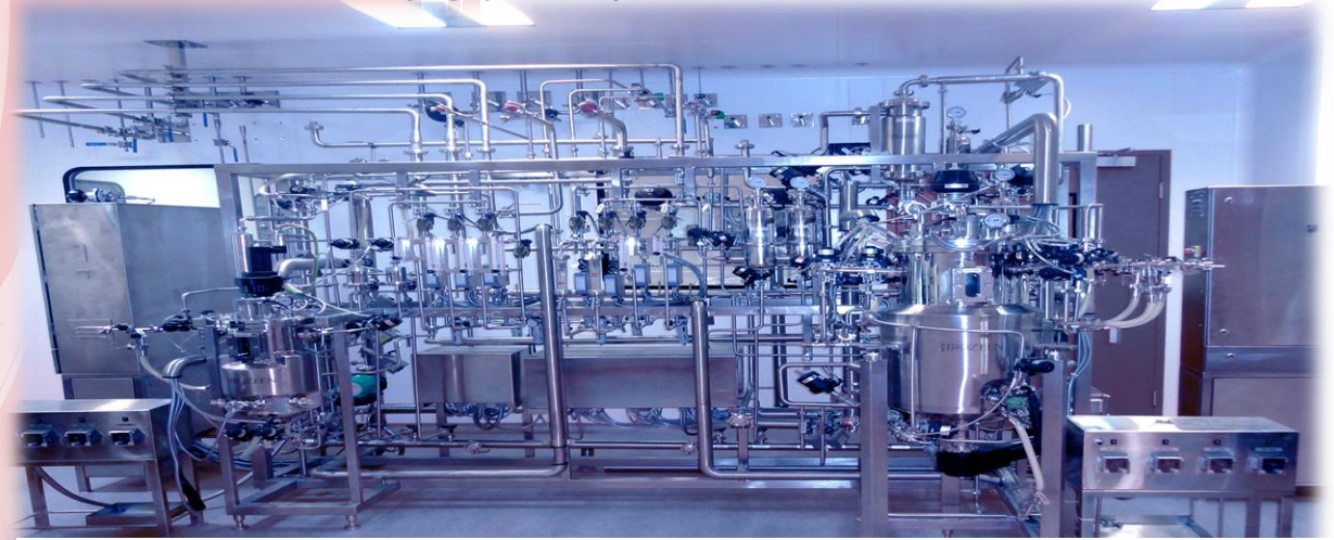
Scale V : Pilot Scale Plant in-situ sterilizable Bioreactor System (50L)
