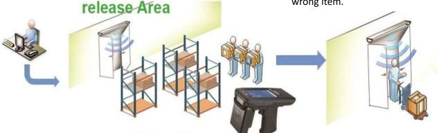
RFID mobile used by operator to search, scan and change status of goods to be sent.
