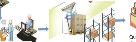
Operator does tagging goods and synchronizes the tags with goods using the RFID Dongle, then saves to Microsoft Dynamic ERP system
