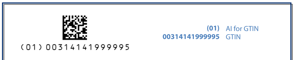
Figure 4: GS1 DataMatrix encoding GTIN – no lot number
