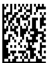
Figure E.3 – Example of GS1 DataMatrix symbol encoded with GTIN AI (01) and Lot Number AI (10).
