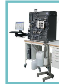
Purification chromatography ÄKTA™ pilot Sephacrose™ 6 Fast Flow size exclusion chromatography
