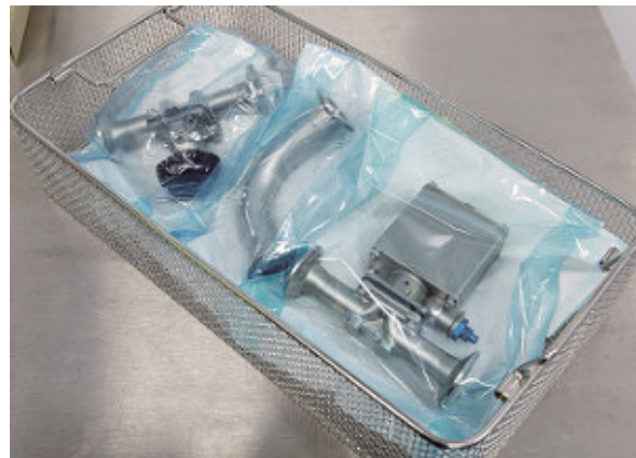
Packing and sealing of goods in steam-permeable bags
