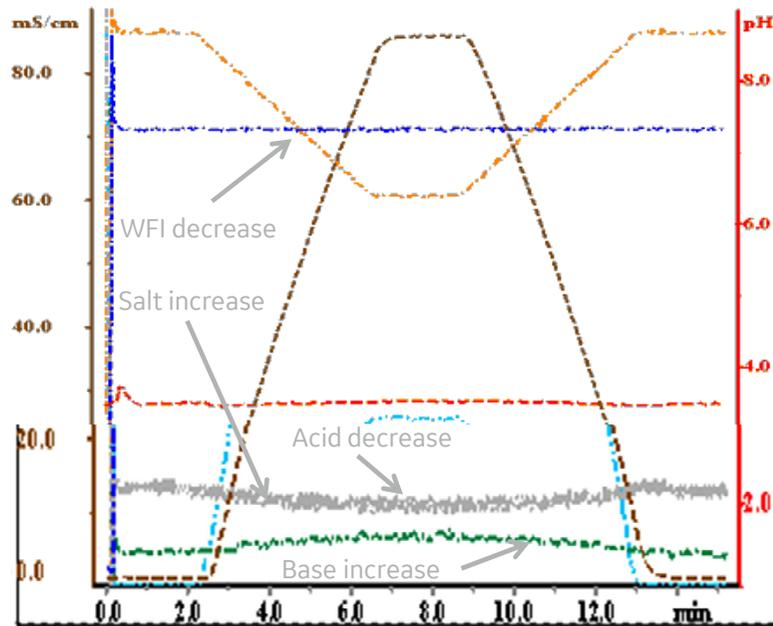
A four-pump solution allows constant pH along the gradient
