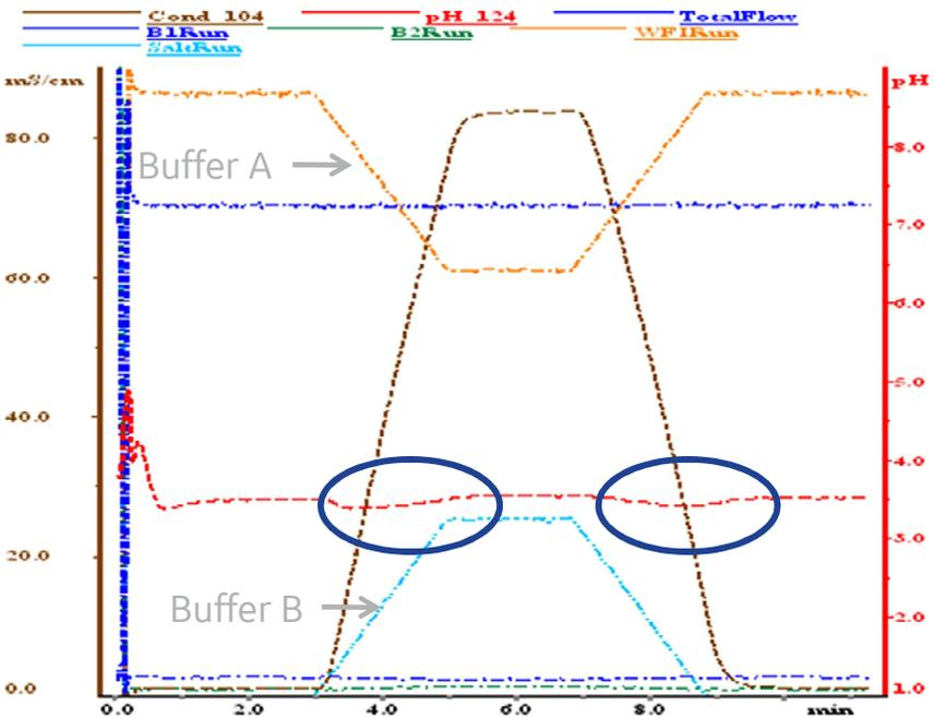
A two-pump solution leads to pH variations along the gradient
