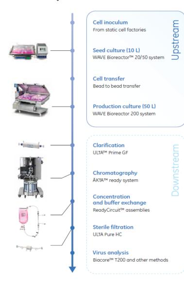
Scale-up from small scale to pilot scale in single-use format
