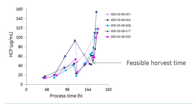
A feasible time for harvest is before the HCP peaks, to facilitate downstream processing
