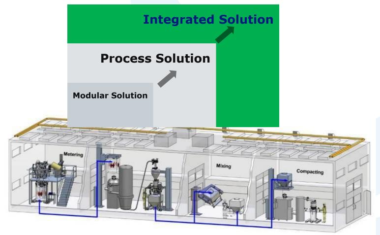
Process planning for a multi-purpose pharmaceutical OSD manufacturing plant
