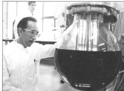
The "Biltoven Unit," designed by the Dutch microbiologists van Hemert (pictured) and van Wezel, generated large quantities of poliovirus for vaccine production in the 1960s.
