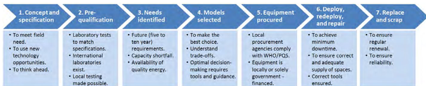
Figure 2. Process of equipping the cold chain from concept to disposal
