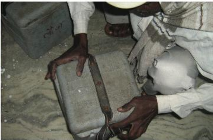
Lid is not airtight which creates temperature control issues
