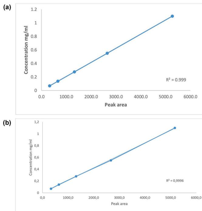
**Fig. 2.** Calibration curve with 2-PE standard on Waters Symmetry 300 column (A); linearity of analytical procedures (B).
