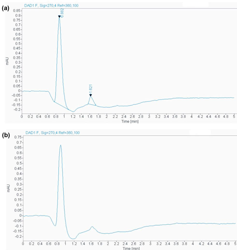
Fig. 3. Chromatogram of one of three independent replicates of the 2-PE concentration  $1.3 \times 10^{-4}$  mg/mL (A) and of the 2-PE concentration  $6.7 \times 10^{-5}$  mg/mL (B).
