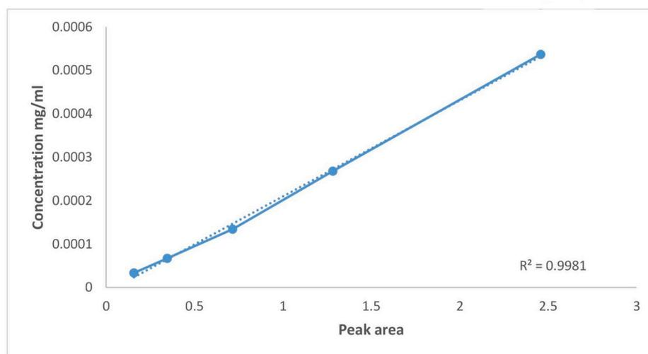
Fig. 4. 2-PE calibration curve for the LOQ determination.
