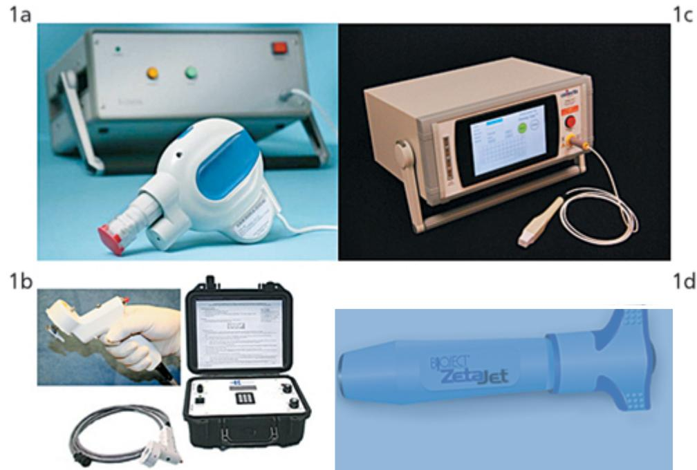
Devices for plasmid DNA delivery including (a) **TriGrid** and (b) **CELLECTRA** with applicator (for intramuscular electroporation), (c) **DermaVax** (for transdermal electroporation) (1d) needless injection device
